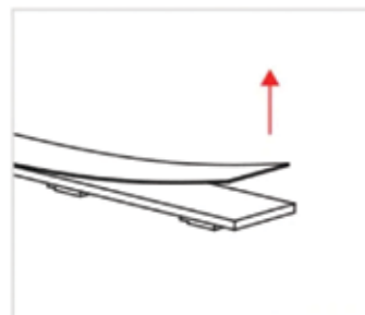
1. Remove the double-sided tape of the light strip
